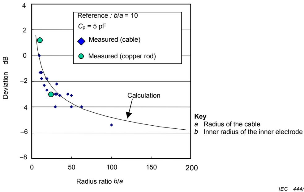
NOTE Vertical axis shows the deviation of the voltage division factor ( $F_a$ ) from the calculated value when  $b/a$  is 10.
