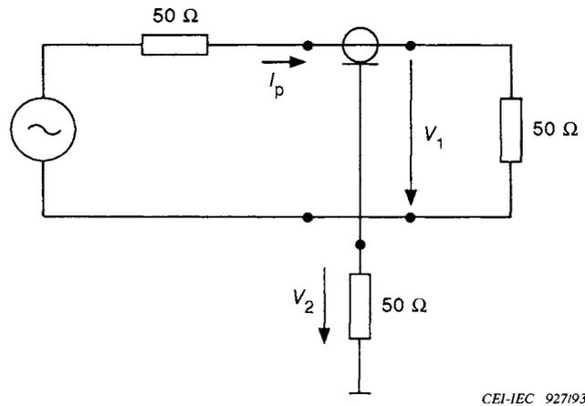
**Figure B.6 – Schematic diagram of circuit with coaxial adapter and current probe
