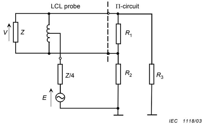
NOTE When terminated with a minimum LCL Π-circuit consisting of  $R_1$ ,  $R_2$  and  $R_3$  ( $R_2 = R_3$ ) which include both the nominal symmetric impedance  $Z$  ( $= \frac{R_1 \cdot (R_2 + R_3)}{R_1 + R_2 + R_3}$ ) of the AAN and the asymmetric impedance of  $150 \Omega$  ( $=$
