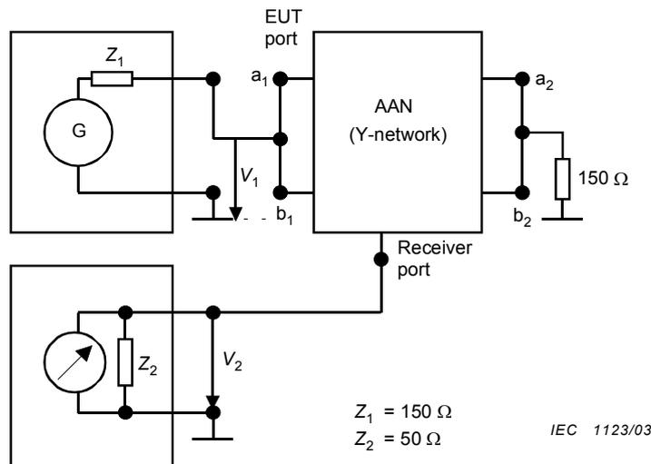
NOTE If the AAN is of higher order (i.e. more than one pair of wires), then all wires of the EUT port respectively all wires of the AE port are connected together.
