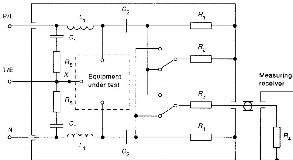
**Figure 5 – Example of artificial mains V-networks,  $50 \Omega/50 \mu\text{H}$ ,  $50 \Omega/5 \mu\text{H} + 1 \Omega$  or  $150 \Omega$  (see 4.3, 4.4, 4.5 and clauses A.3, A.4 and A.5, respectively)**
