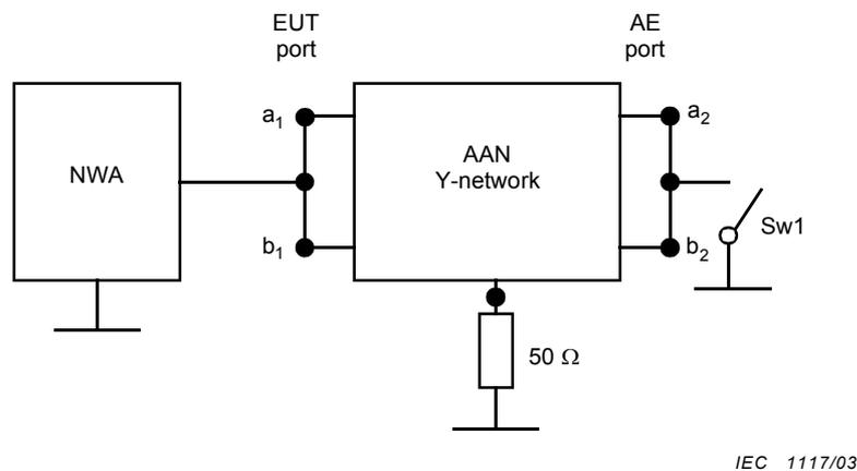
NOTE If the AAN is of higher order (i.e. more than 1 pair of wires), then all wires of the EUT port, respectively all wires of the AE port, are connected together.
