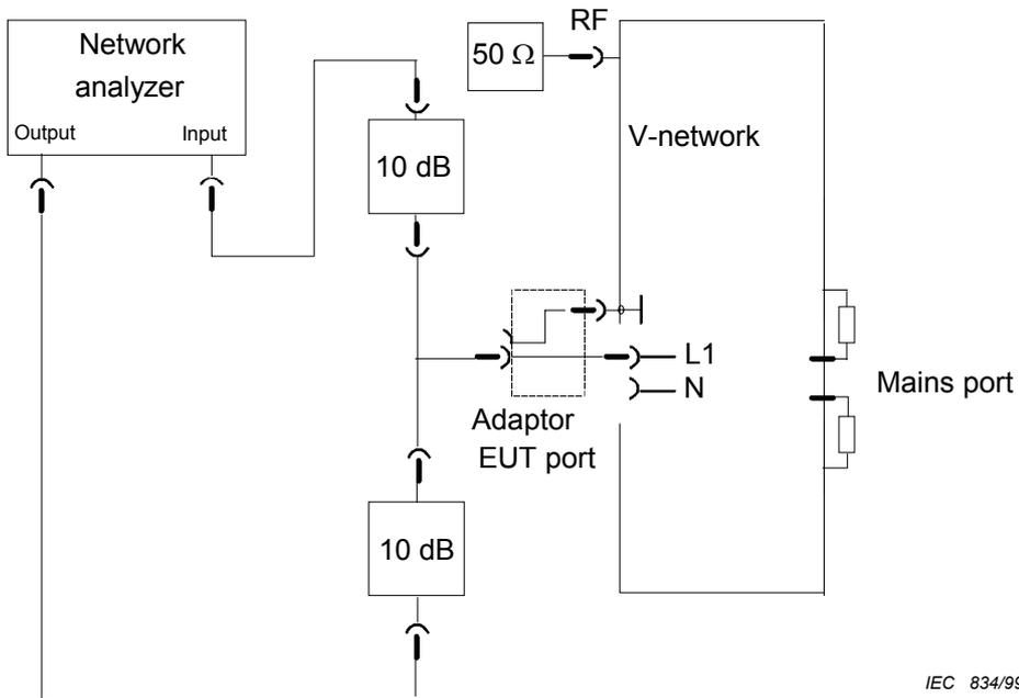
**Figure A.6a – Test set-up for normalization of the network analyzer**
