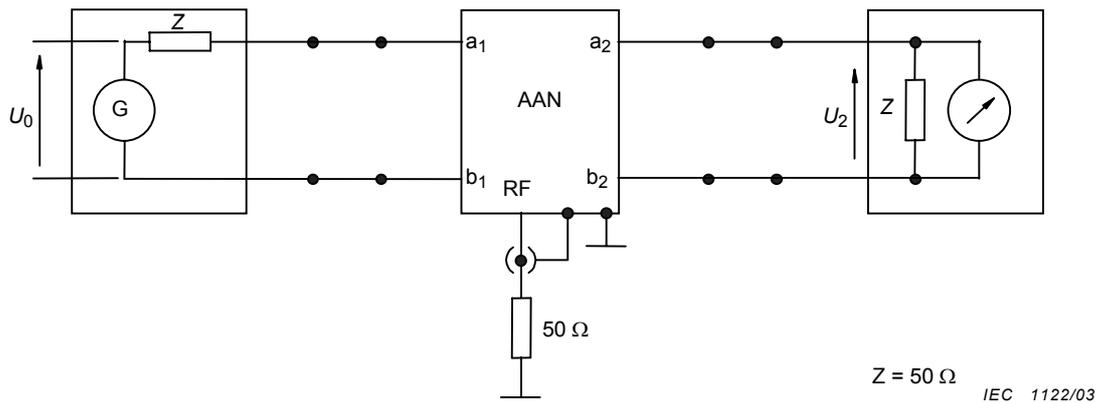
The decoupling attenuation specification shall be met in both positions of Sw1 (short and open). If the AAN is of higher order (i.e. more than 1 pair of wires), then all wires of the EUT port respectively all wires of the AE port are connected together.  $a_{vdiv}$  is the voltage division factor as measured in accordance with Figure E.6.
