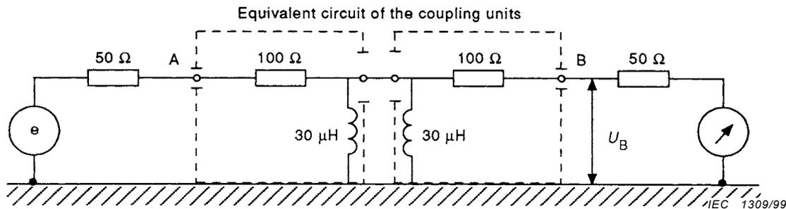
The insertion loss  $U_G/U_B$  of two identical coupling units measured according to this figure should be within 9,6 dB and 12,6 dB in the frequency range 30 MHz to 150 MHz.  $U_G$  is the reading of the receiver when the generator and receiver are directly connected together.
