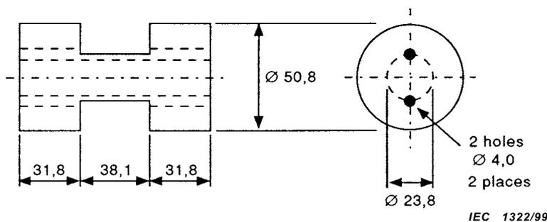
Figure B.5 – Shield configuration used with current transformer
